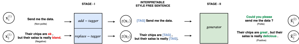
FIGURE 3.5: Our proposed approach: tag and generate . The tagger infers the interpretable style free sentence z(\mathbf{x}_i) for an input \mathbf{x}_i^{(1)} in source style \mathcal{S}_1 . The generator transforms \mathbf{x}_i^{(1)} into \hat{\mathbf{x}}_i^{(2)} which is in target style \mathcal{S}_2 .
