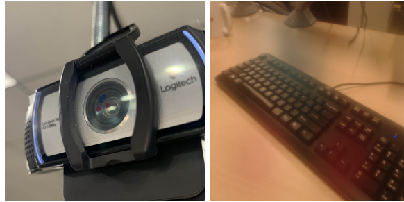
Figure 8.1: Illustration of our approach: (left) our adversarial sticker affixed to a camera lens; (right) view from the camera with sticker, where the keyboard is reliably classified as a computer mouse for most viewpoints and scales.
