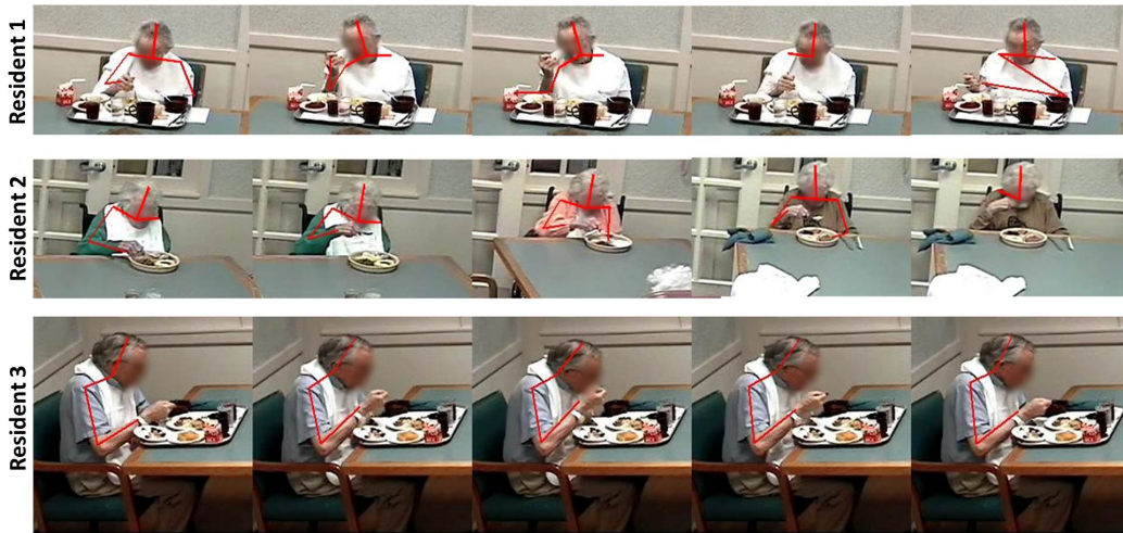
FIGURE 6.5: Snapshots of pose estimation for eating residents. Success and failure cases are both shown.
